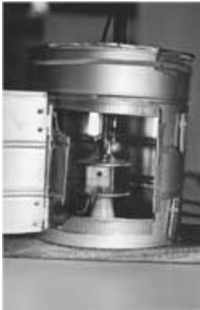
Close-up of the homemade neutralizing capacitor assembly built inside a coffee can. The sample is placed between the two parallel plates. (Roger Ham)
